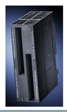
SIMATIC S7-300 digital input SM 321, Isolated in groups of 16, 64 DI, 24 V DC, 3ms, Sink/source input Terminal blocks 6ES7392-1.N00-0AA0 and cable 6ES7392-4...0-0AA0 required
