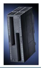
SIMATIC S7-300 digital output SM 322, Isolated in groups of 16, 64DO, 24 V DC, 0.3A sink output Total current 2 A/group, 8 A/module Terminal blocks 6ES7392-1.N00-0AA0 and cable 6ES7392-4...0-0AA0 required
